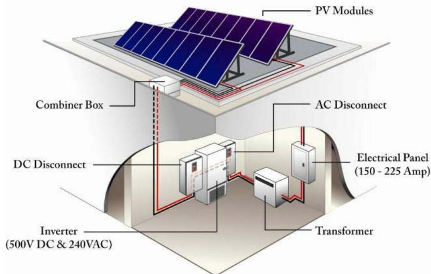
**Figure 1. Major components of grid-connected photovoltaic (PV) system**
